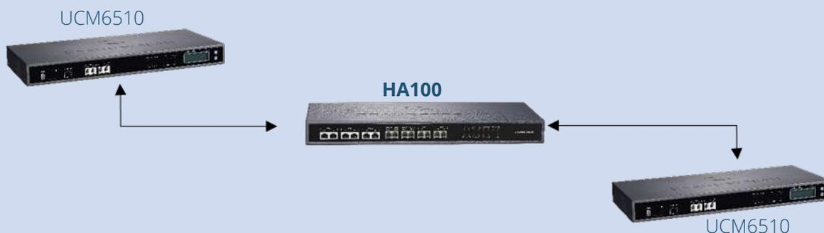
The HA100 is ideal for any business that requires an always-on, redundant voice system by providing an automatic failover solution when paired with two UCM6510 IP PBXs. The HA100 constantly monitors the operational status of both UCM6510s and automatically switches all system control to the hot-standby secondary UCM6510 in the event that the primary device fails. It can complete the entire system switch between 10 and 50 seconds depending on the number of registered SIP endpoints.
